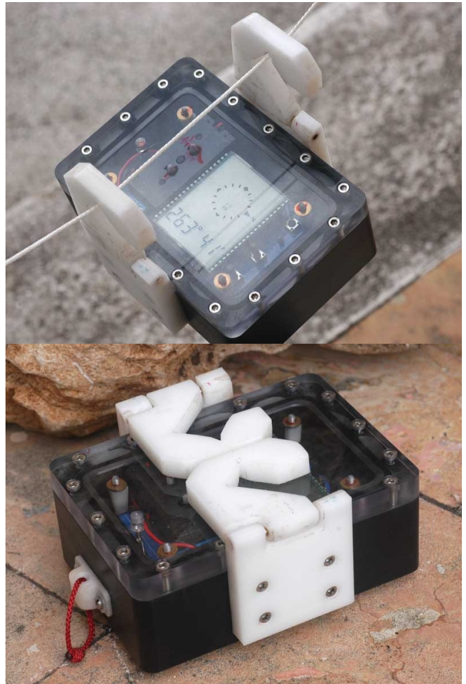
Figure 3: Compass suspended on line hangers (top). When not in use, hangers fold flat against compass body for stowing in pocket (bottom).
