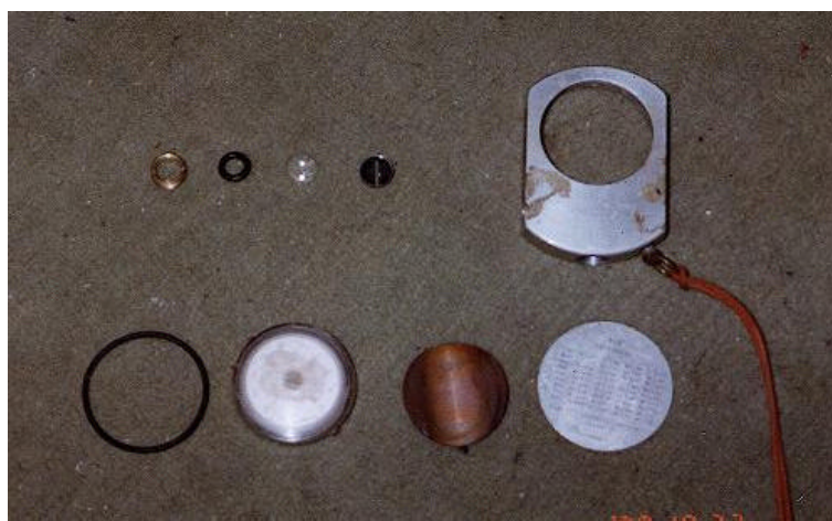
Figure 2 - The completely disassembled instrument. The top row is bush, O-ring, lens, sighting slot, body. The bottom row is O-ring, capsule, Spring-washer, Backplate
