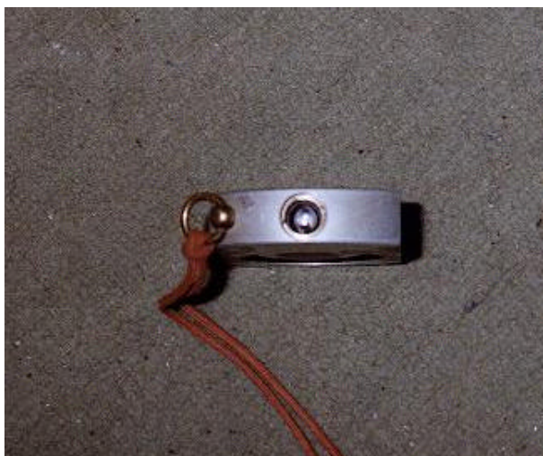
Figure 1 - The finished item, with the ring replaced by a removable bush.
