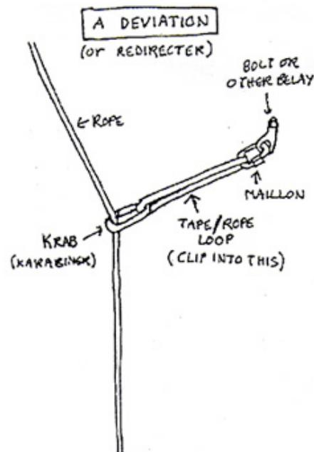
A deviation (or redirecter) is another means of avoiding rub points and other hazards by altering the hang of the rope down the pitch. The rope runs freely through a krab which is attached to a belay via a tape or rope-loop. This deviation pulls the rope away slightly from its natural vertical hang to move the rope below the deviation away from a rub-point. A deviation never bears the full weight of a caver (or a fraction of it) and consequently
