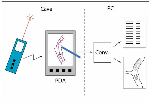
Fig. 1: Data flow from measuring device via PDA and converters to PC based cave applications.
