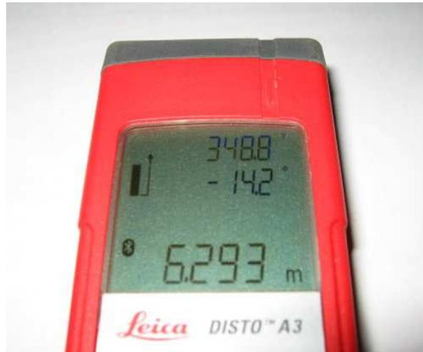
Fig. 2: Leica Disto with compass and clinometer readings added to the standard display.
