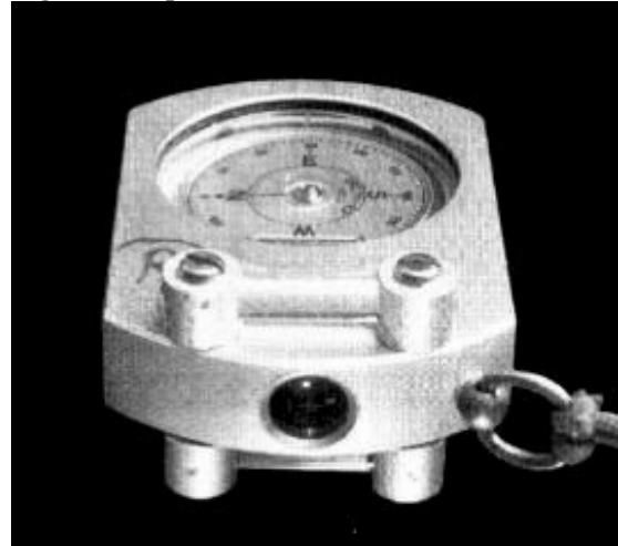
Fig.1: SUUNTO Compass with mounted Plexiglas cylinder. The light received from the opposite survey point shows as a vertical line in the Plexiglas cylinder and enables a correct bearing, even in steep sections. This system eliminates inexact guesses of the vertical extension when taking the compass bearing. Such errors can be unbelievably huge on steep routes (over 30° inclination). Detailed description and how to assemble this system are found in Weissensteiner und Trüssel (1991) or www.speleo.ch/equipment . Photo M. Trüssel.
