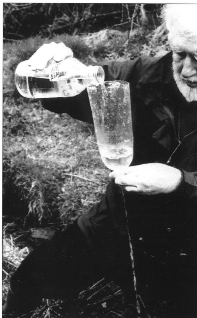
Figure 2.1. Measuring the discharge of St. Cuthbert's Stream by standard addition
