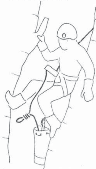
Fig.3. Self-protection while rigging a traverse line.
