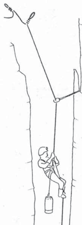
Fig.11. "Deviation" technique.
