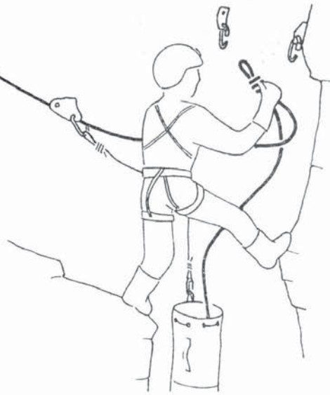
Fig.2. Self-protection while rigging the main belay.
