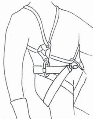
Fig.11. Optional use of chest harness for self-lifeline with certain jammers.
